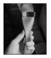
7. For the first row rear seat, stow the safety belt latch by attaching the clip on the safety belt latch to the trim just inside the side door. For the remaining rear seats, stow the safety belt latch plate on the clip at the window trim.
